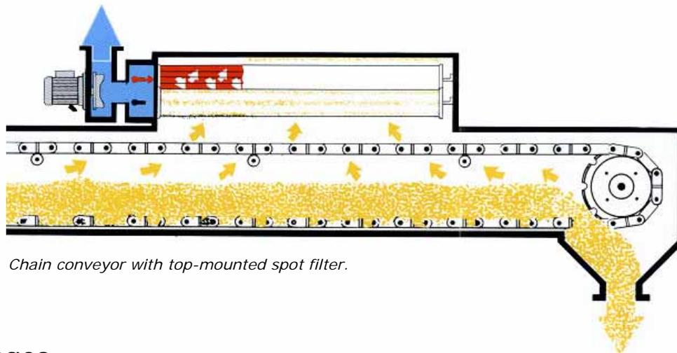
*Chain conveyor with top-mounted spot filter.*
